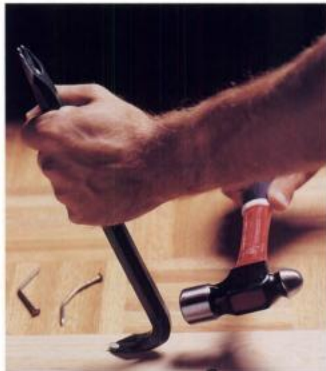
A cat's paw has a sharpened claw for removing stubborn nails. Use a hammer to drive the claw into the wood under the nail head, then lever the tool to pull up the nail.
