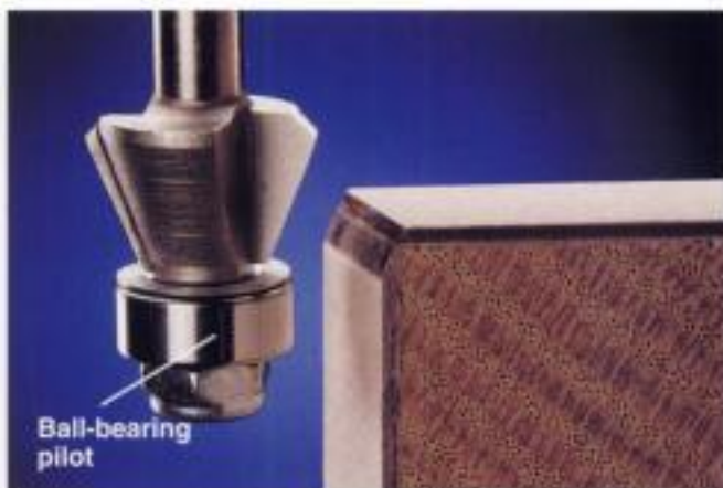
A laminate trimmer bit cuts a finished edge on plastic laminate installation. A ball-bearing pilot prevents the bit from scorching the face of the laminate.
