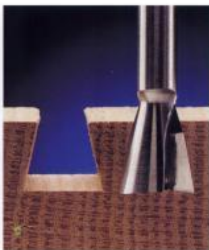
A dovetail bit cuts wedge-shaped grooves used to make interlocking joints for furniture construction and cabinetwork.
