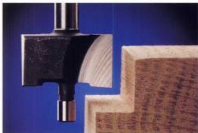
A rabbet bit makes step-cut edges. Rabbeted edges are often used for woodworking joints and for picture frame moldings.
