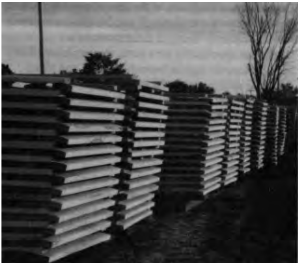
Missouri staves stacked for dry kiln. Photo courtesy of McGinnis Wood Products, Inc. (SFP-4)
