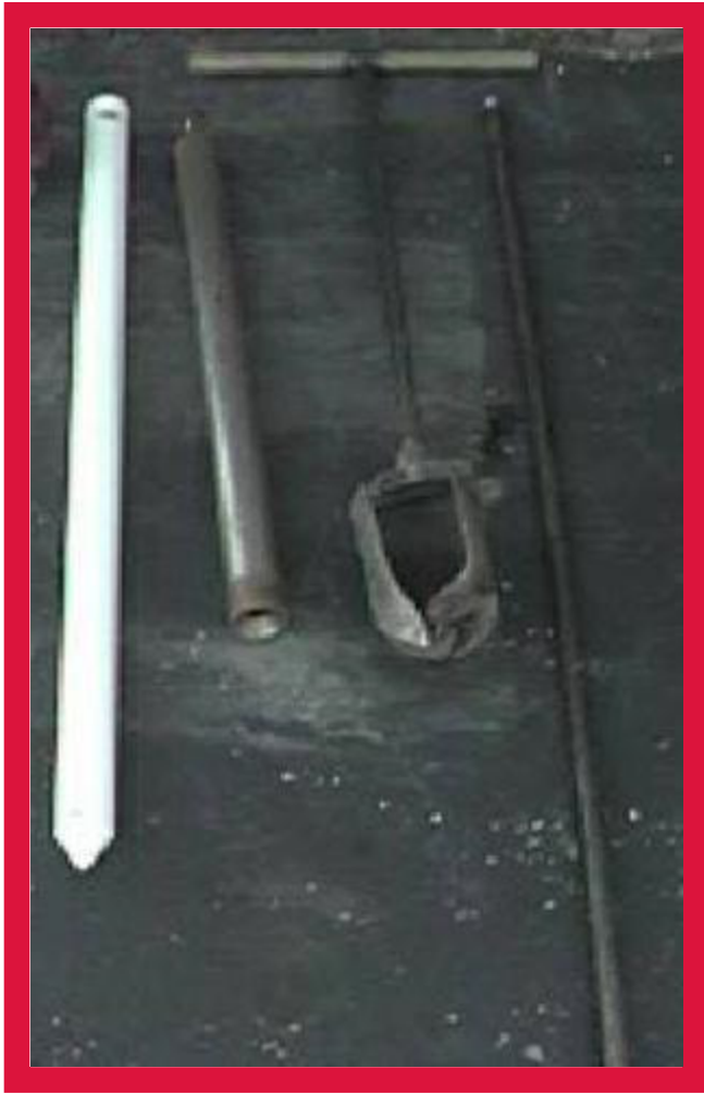
LEFT PHOTO: PVC drivepoint RIGHT PHOTO: drivepoint, sand sucker, auger, and auger extension
