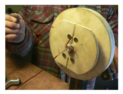
Drop the wire in the slot of the coil winder and bend the end around the nut. (A wing nut helps here too..) This will hold the wire from slipping when you wind the coil.
