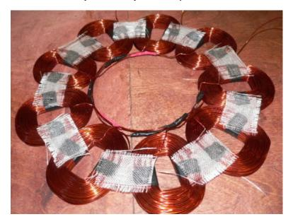
Now you can carefully pick up the uncast stator and remove it from the mold. Put it somewhere safe untill you're ready to cast the stator in resin.
