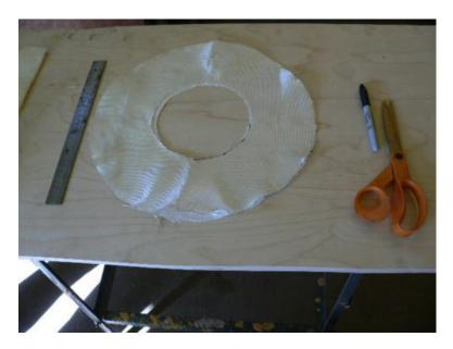
In the picture you can see the two rings of fiberglass. Set them, and the coils aside for now. Grease the stator mold inside, on top - and around the edge. Same with the lid - everything should be carefully covered with grease, or wax. Automotive or wood wax works really well.
