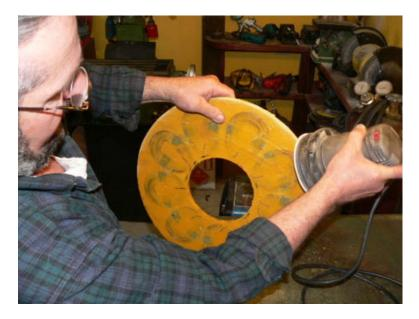
Use a file or a sander (or both) to clean up the edges of the stator. The inside diameter must be pretty clean because there's not a lot of extra room between this hole and the wheel hub which will exist inside it.
