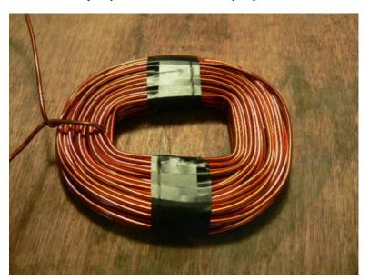
We refer the longest sides of the coil as the 'legs'. Tape the legs of the coils with a couple wraps of electrical tape to hold things together. One coil is finished.
