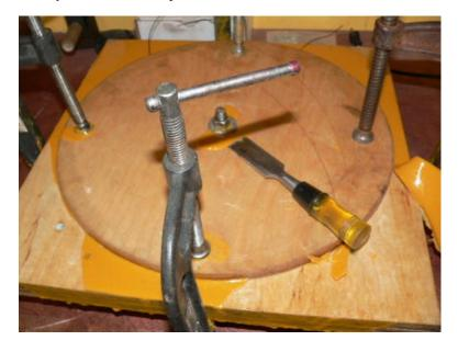
A chisel works well to scrape/peel the resin off around the outside of the mold. A good time to do this is while it's still a bit flexible (before it gets really hard).
