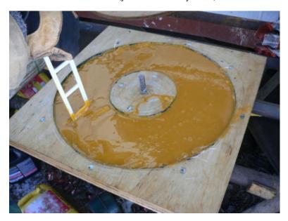
Then pour about another pint of resin in the mold, work it into the fabric more - try to work out any airbubbles.
