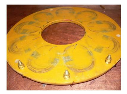
The stator is finished! We can put that aside untill we're ready to assemble the alternator.
