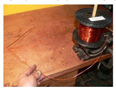
About 10" from the end of the wire bend it sharply 90 deg with the needle nosed pliers.
