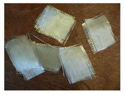
Cut 9 little rectangles from fiberglass cloth about 1.5" wide and 2" long. Before you cast the stator you'll need to remove the coils from the mold again. We'll use these squares of cloth and superglue to hold everything together so that we can move it.
