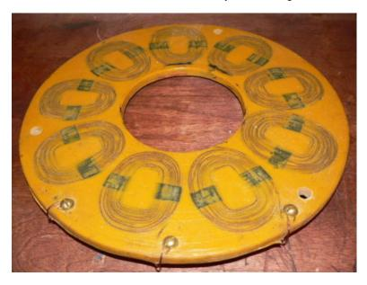
Insert a brass 1/4 - 20tpi screw through each one, with a washer on each side and a nut on the back. Cut the leads just long enough so you can clamp each one between a screw head and the washer. You can put a couple more washers and one nut on each screw now. These will serve as the lugs to which we can connect the line to the wind turbine.
