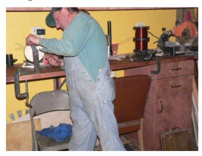
Pictured above Scott's winding with two strands of wire. This is necessary for 12 Volt machines.
