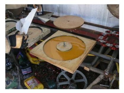
It takes about exactly 1/2 gallon of resin to cast the stator. Find a level place to put the mold. It's important to either keep the edges of the mold off the workbench - or find a work bench (like the one in the picture) that allows access for C clamps around the edges of the mold. When your done you'll need to clamp the lid down with C clamps so think ahead! Pour about a pint of resin into the mold and roll the mold around so that the whole bottom and the sides become covered 'wet' with resin.
