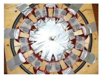
In the picture you can see all the coils are connected to one another with fiberglass cloth.
