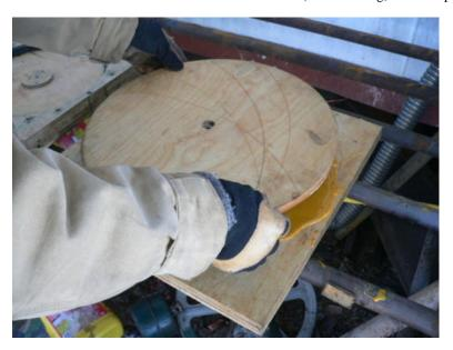
Carefully put the lid of the mold down over the casting.
