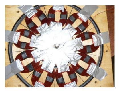
Even though the coils fit well and are the right size, once we make all these connections things are kind of springy and surely the coils are not in their perfect place. The connections we made and all that wire around the inside is sure to push some of the coils out further than they ought to be. Use duct tape and go around the stator 1 coil at a time, and tape it exactly where it belongs. Keep the tape off the 'legs' of the coils as shown in the picture.
