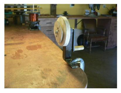
Clamp the coil winder to the workbench with a C clamp as shown in the picture.
