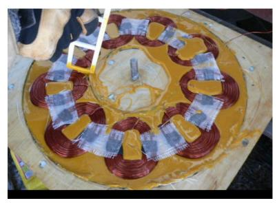
Put the coils in carefully, poke at them so resin runs all around the coils and airbubbles come up.
