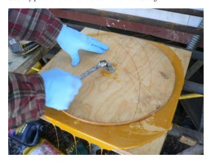
Put a 1/2" washer over the threaded rod, and run the 1/2" nut down over it. Tighten the nut - this does a good job of clamping the lid tightly on the mold and assuring that the finished casting will be 1/2" thick.
