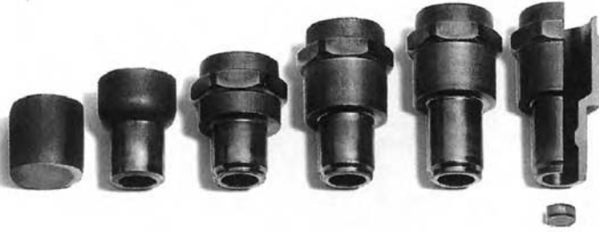
Figure 27.17 Sequence of operations for a spark plug barrel produced on a Coldmatic transfer press (Photograph from Hatebur works, Reinach, Switzerland)
