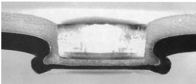
Figure 20.2 Cross-section of a joint clinched using movable die segments; connecting aluminium (above) and steel (below) (Fraunhofer Institute for Machine Tools and Forming Technology, IWU, Chemnitz, Germany)
