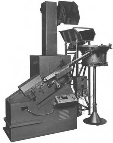
Figure 6.10 Automatic high-performance thread rolling machine, type R 2 L (Photograph from Hilgeland works, Wuppertal, Germany)
