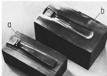
Figure 7.2 Forging die for cutlery handle, a) hub, b) hubbed stamping die
