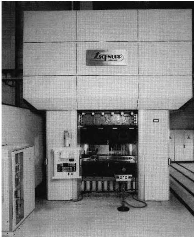
Figure 14.35 Schnupp sheet hydroforming press at the AUDI AG company (Photograph from Schnupp GmbH & Co Hydraulik works, 94327 Bogen, Germany)
