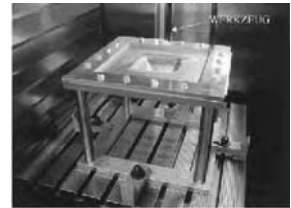
Figure 15.9 Test facility in Hermle C 500 V HSC milling machine
