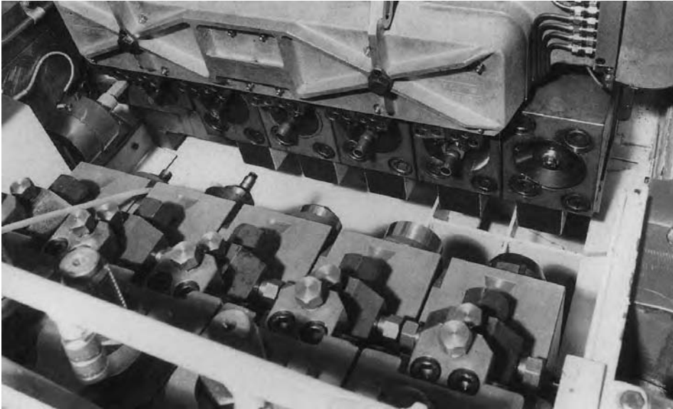
Figure 27.14 Tooling area of a transverse feed transfer press (Photograph: Hatebur works, Reinach, Switzerland)
