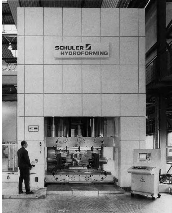
Figure 14.40 50,000-kN tube hydroforming press at the Fraunhofer Institute for Machine Tools and Forming Technology in Chemnitz (Photograph: Schuler Hydroforming GmbH & Co. KG works)
