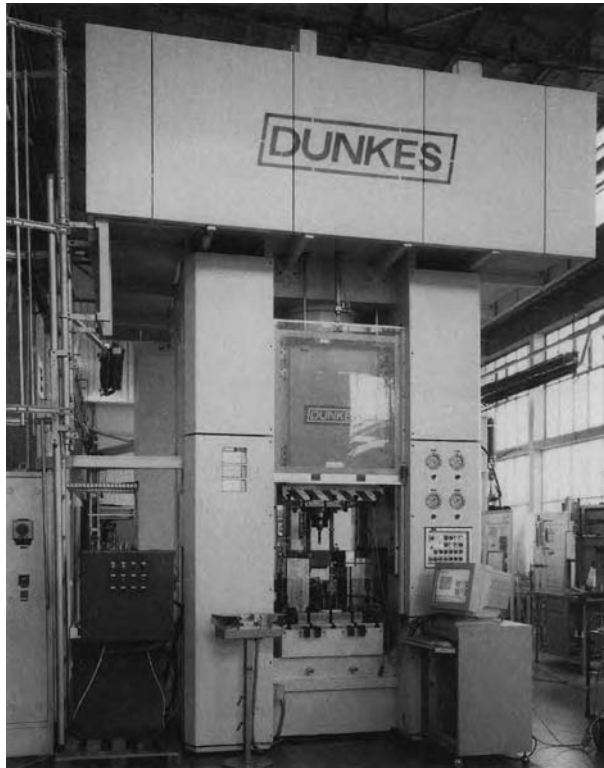
Figure 26.6 Hydraulic double-sided extrusion press (Photograph: Dunkes GmbH works, Kirchheim unter Teck, Germany)
