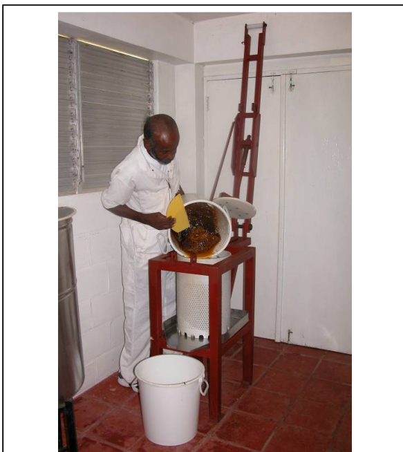
Picture 6 Honey press being used by Gladstone Solomon. The press was designed and built as part of the Project.
